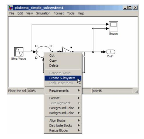
Optionally, rename In1 and Out1 to U and Y respectively. This operation results in a subsystem like the following:
