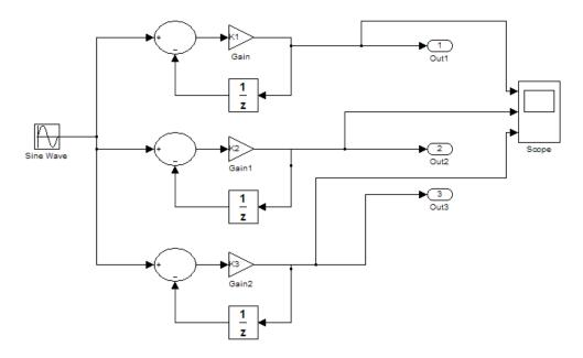
2 Select the Sum, Gain, and Unit Delay blocks and create an atomic subsystem with inputs U, U1, and U2 and outputs Y, Y1, and Y2. Rename the Subsystem block as SimpleSubystem. When you are finished, the top model and atomic subsystem model should look like the following:
