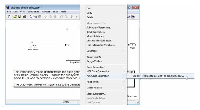
This command opens the block parameter dialog box so that you can select the **Treat as atomic unit** check box.
